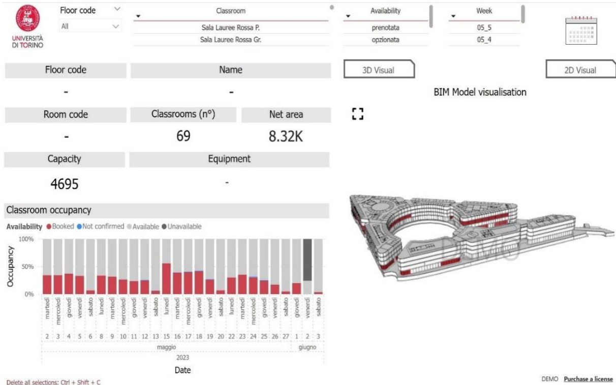
Figure 10: AMS-App dashboard facilitating the analysis of lecture hall spaces availability and occupancy at the building level with 3D visualization.
