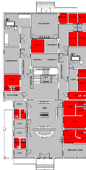
Figure 7: Hospital ground floor with grey showing the allowed regions and red showing the restricted regions.
