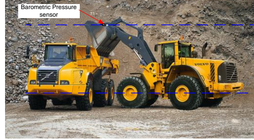
Figure 6 –Pressure Sensor Attached to Loader Bucket
