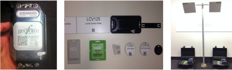
FIG. 9: The demonstration of portable RFID system: GPS tags, passive tags, readers and pole antennas
