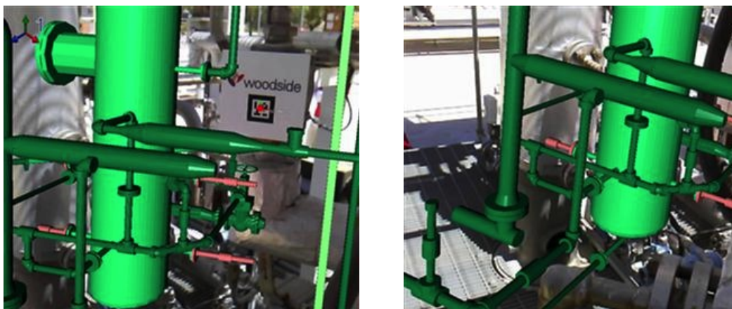
FIG. 14: Display of AR assembly context: a) marker tracking; b) 3D feature tracking.
