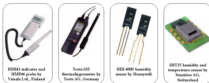
FIG. 2: Examples of relative humidity and temperature measurement devices (Voutilainen, 2005).
