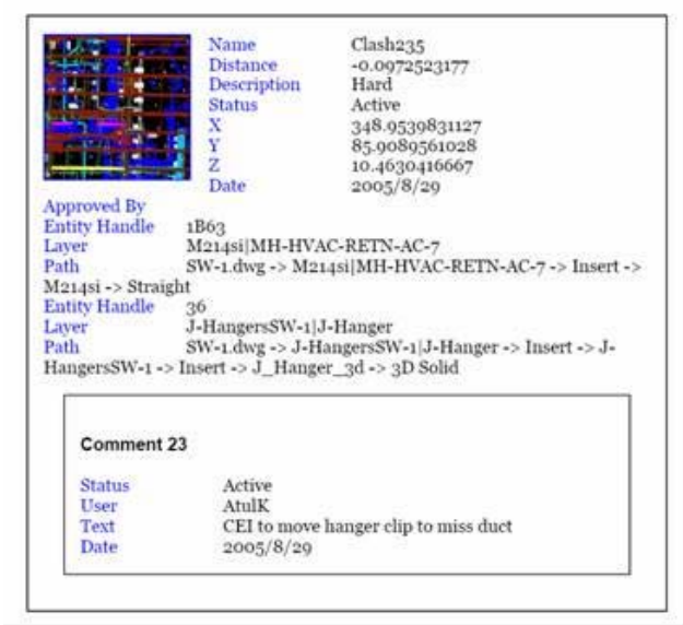
FIG. 11: Conflict identification and resolution report from the Camino Project generated directly from Navisworks Clash Detective.
