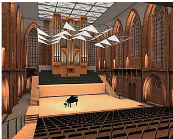
FIG. 18: Models to integrate visual and aural features. Pekka Salminen's Marienkirche concert hall renovation in Neubrandenburg, Germany 1996-2001. Visual combined with acoustic modelling, spatial characteristics can be simulated.
