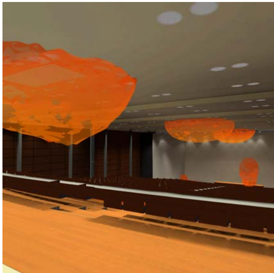
Fig. 7: Isosurfaces near ventilation illustrating velocity of airflow in Hall 600.
