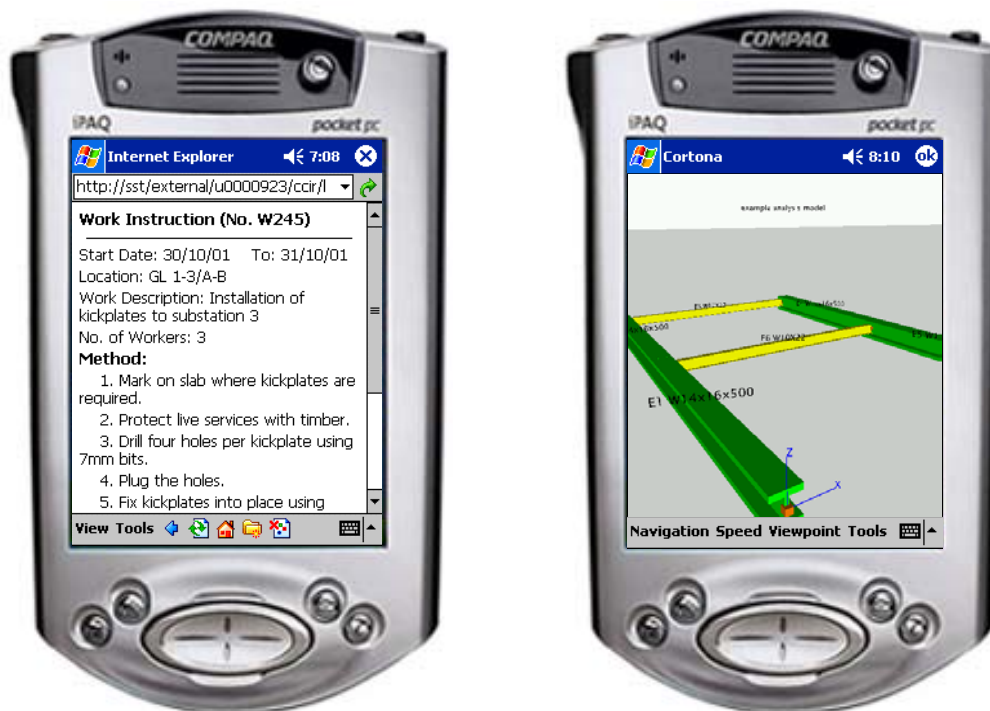
FIG. 11: Work instructions and assembly VR model via Pocket PC.
